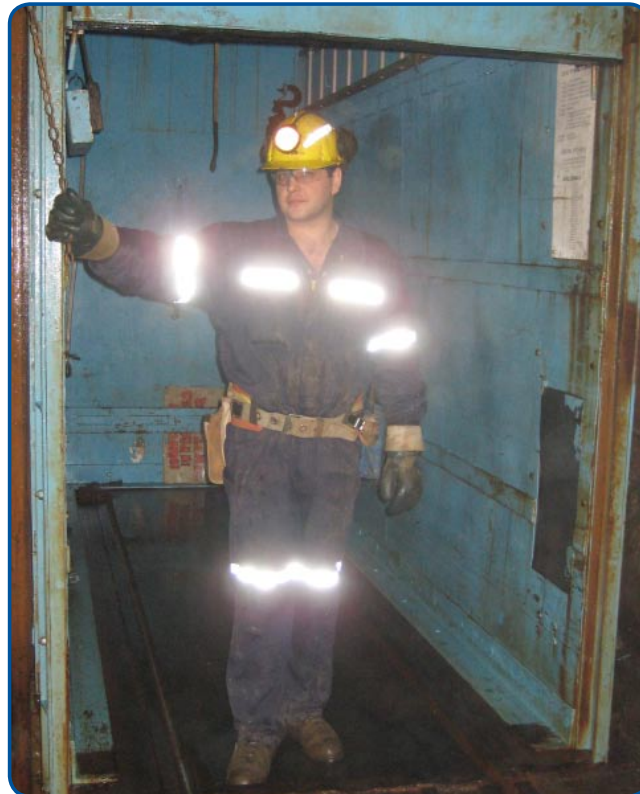
Figure 2: Cage Tender Signalling the Hoistman
