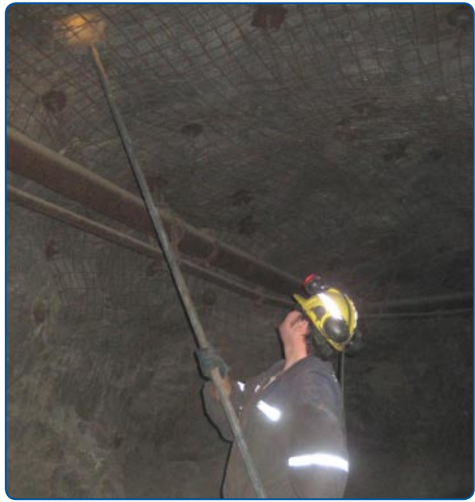
Figure 2: Scaling the Back of a Drift
