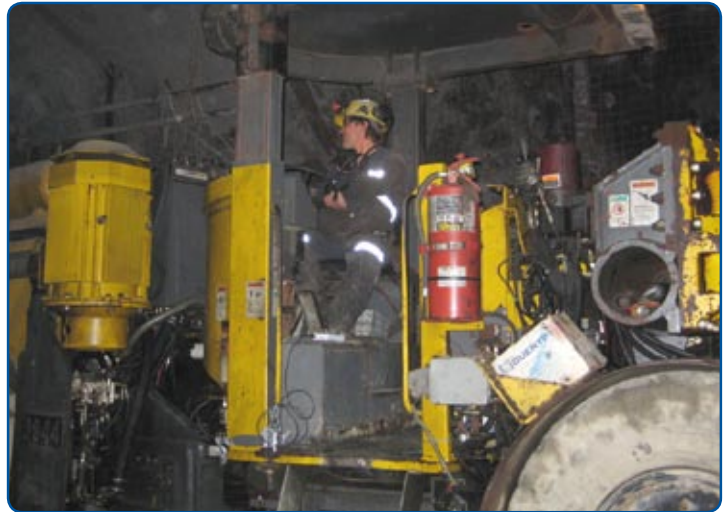
Figure 2: Driving Jumbo Drill
